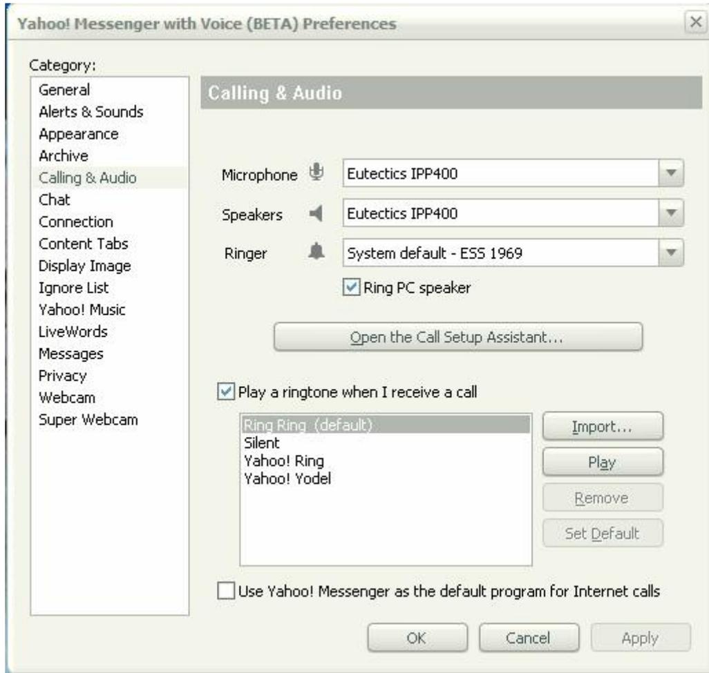
3. Set the Audio In and Audio Out to the Eutectics device id (IPP400 or any of the IPP Internet Power Phone devices). On windows 2000, ME or 98 this will be USB Audio rather than a specific device name
